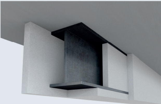
Beam with open profile.
