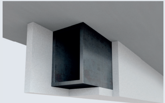
Beam with closed profile.
